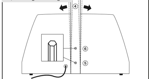
Align the rod (4), first tighten the lower screw (5), then tighten the upper screw (6).
