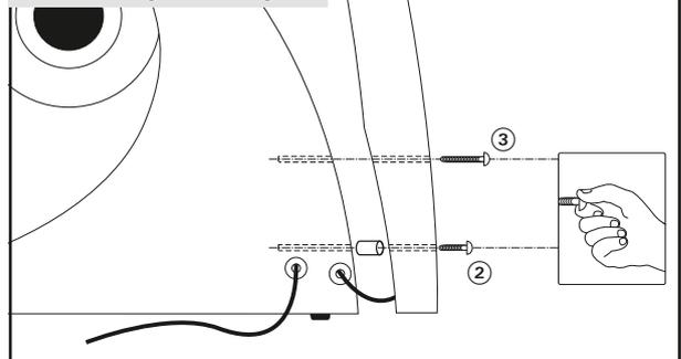
Set up the rod, insert the lower screw (2), slide on the sleeve and tighten the screw hand tight. Screw in the upper screw (3) and tighten it hand tight. Attention: Ensure that the cable is not pinched in the rod!
