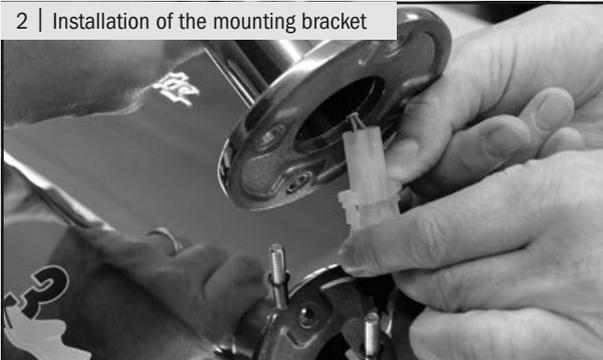
First remove the four hexagon cap nuts M6 and the spring rings from the housing of the shoe polishing machine using a spanner. Person 1 holds the mounting bracket vertically over the shoe polishing machine. Person 2 connects the plug of the shoe polishing machine with the plug connector of the mounting bracket. Make sure that the catches lock in.
