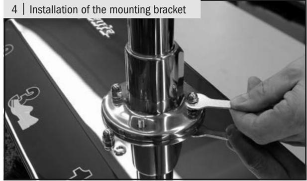
Place four spring rings on the threaded bolts, and tighten each with a cap nut using wrench.
